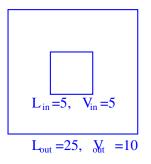
Use a relaxation method to compute the potential distribution between the two concentric square cylinders shown in the figure. The potential and the length of the square are given in the figure. Sketch the equipotential surface.
