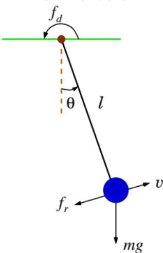
A point mass  $m$  is attached to the lower end of massless rod of length  $l$ . The pendulum is confined to a vertical plane, acted on by a driving force  $f_d$  and a resistive force  $f_r$  (see the figure). The motion of the pendulum is described by Newton's equation along the tangential direction of the circular motion of the mass,
